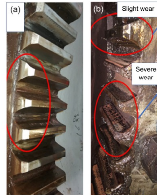
Fig. 17 Wear of gears in a wind turbine.
